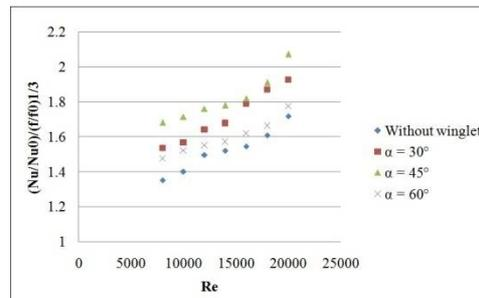
Fig. 5. Thermal performance vs Re for P 20mm.
