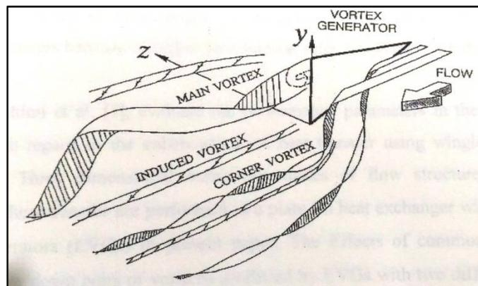
Fig. 1. Vortex system behind a delta winglet [1].
