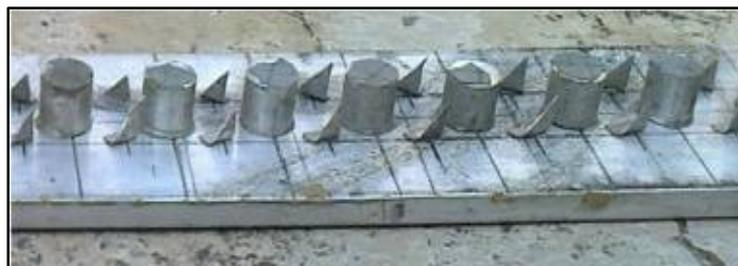
Fig. 3. Pin fins with Delta winglet vortex generators
