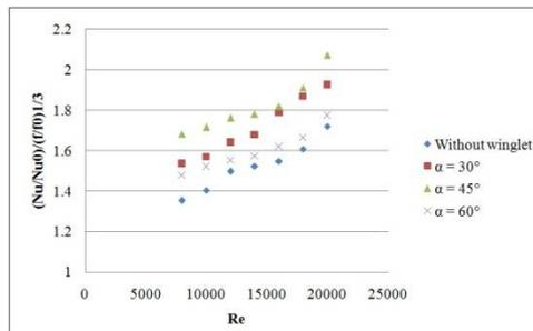
Fig. 6. Thermal performance vs. Re for P 22mm.
