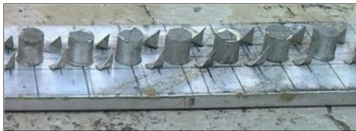
Fig. 3. Pin fins with Delta winglet vortex generators
