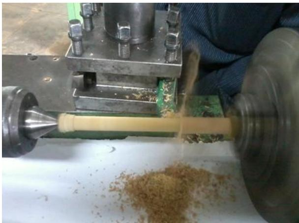
Fig.4 Lantana Camara stem turned in lathe
