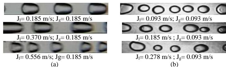
Fig. 4 The bubble flow patterns for (a) the 3 mm x3 mm channel and (b) the 3 mm x 6 mm channel
