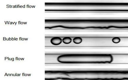
Fig. 1. Huang's flow patterns [1] modified
