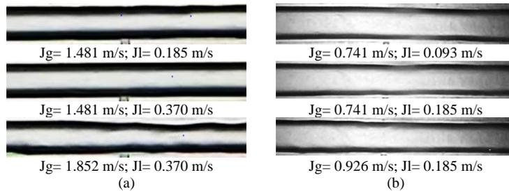
Fig. 6 The annular flow patterns for (a) the 3 mm x 3 mm channel and (b) the 3 mm x 6 mm channel
