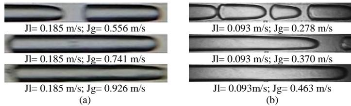
Fig. 5 The plug flow patterns for (a) the 3 mm x 3 mm channel and (b) the 3 mm x 6 mm channel
