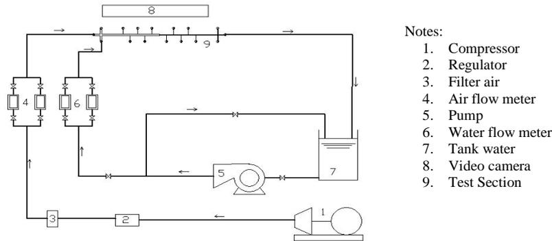
Fig. 2 Schematic view of research tool
