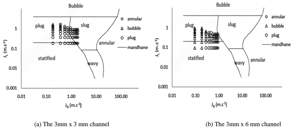
Fig. 7 Flow pattern observation at Mandhane's Flow Pattern Map [3]
