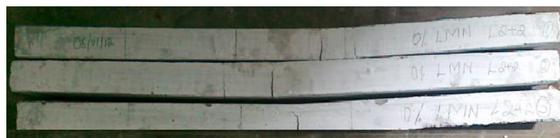
Fig 5 – Failure of Specimens in 0% replacement of BFS
