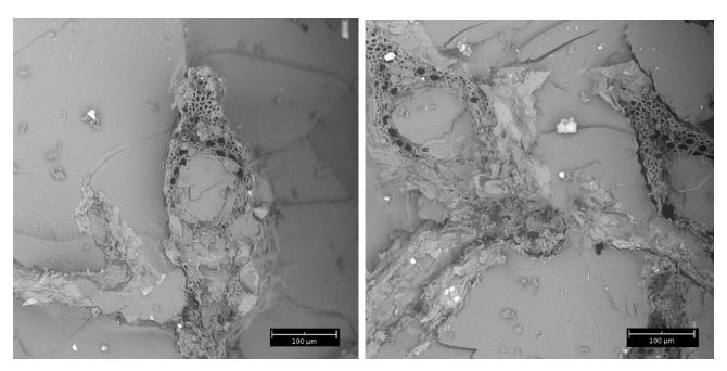
**Figure 4.** Scanning Electron Micrographs of the Fractured Surface of the Combined Alkali-Bleach Treated Mengkuang Cellulose Fiber Composite (500x Magnification).
