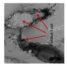
Figure 2. SEM of fractured surface of untreated cellulose fiber Composite Fiber-Matrix a) Crack Formation (200x Magnification) b) Unfilled Holes of the Fiber (500x Magnification).
