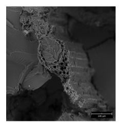
**Figure 3.** SEM Micrographs of fractured surface of the alkali treated cellulose fiber Composite fiber-matrix bonding (500x Magnification) a) Crack Formation b) Unfilled Holes of the Fiber.
