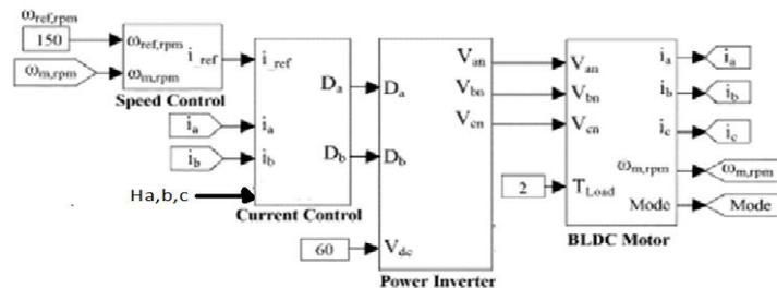
Fig.10.Simulink model of FSTPI-BLDC motor
