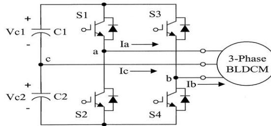
Fig.2. Proposed four switch three phase BLDC motor drive.
