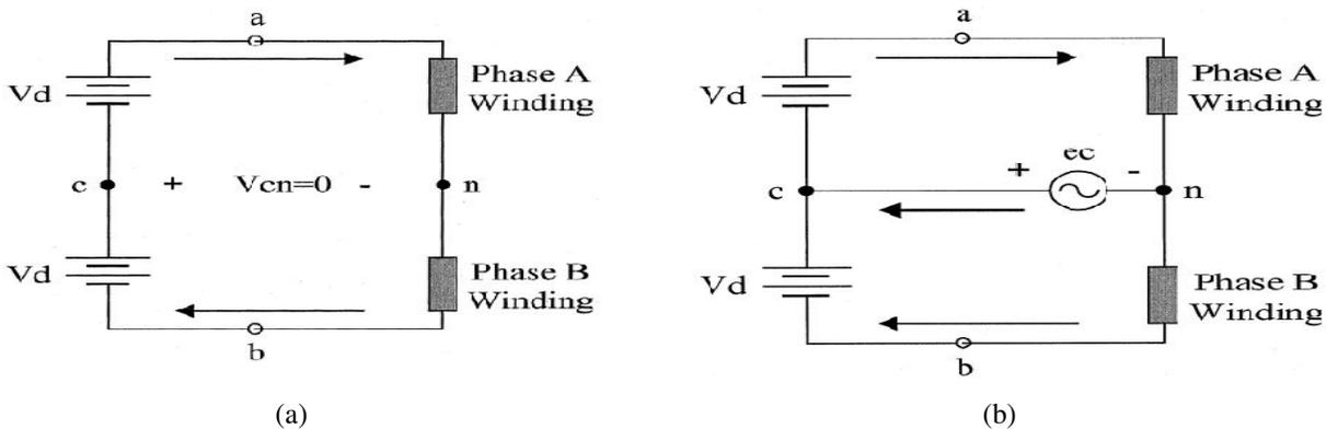
Fig. 8. Simplified circuits showing modes II and V. (a) Ideal case. (b) Effect of back emf of phase C.
