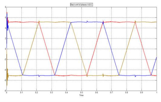
Fig.11.Back emf waveforms of the three phases.
