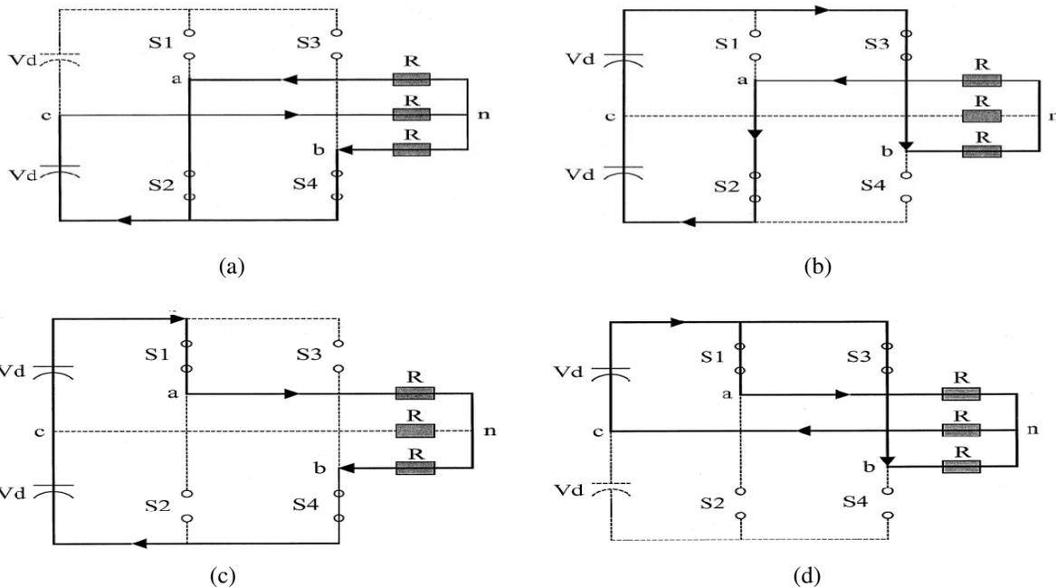
Fig 5. Voltage vectors of four switch converter with resistive load: (a)(0,0) vector, (b)(0,1) vector, (c)(1,0) vector, (d)(1,1) vector.
