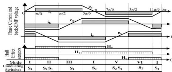
Fig 4. Phase current and trapezoidal back emf of BLDC motor with hall sensor signals.
