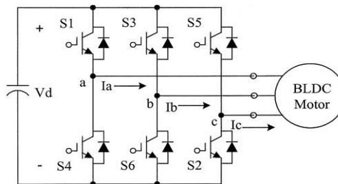
Fig.1 Conventional six-switch three phase BLDC motor drive.
