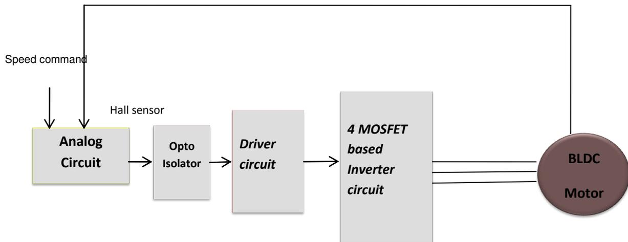
Fig:14. Block diagram of Hardware Implementation
