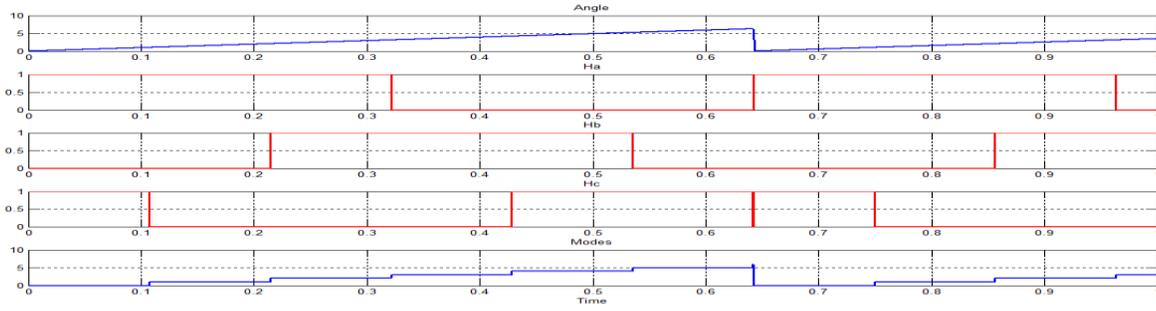
Fig.13.Virtual Hall sensor signals and operating modes.
