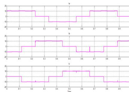
Fig.12. Rectangular phase current waveforms of phases A,B and C.
