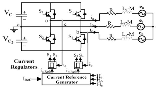
Fig.3. Equivalent circuit of FSTPI BLDC motor drive.
