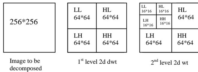
Figure.2. DWT decomposition of an image
