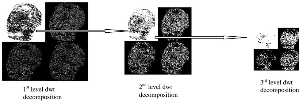
Figure.6. Multi-level DWT decomposition
