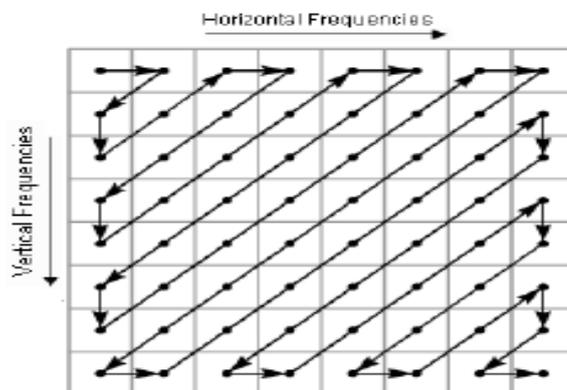
Figure.4. Raster scan order of dct coefficients
