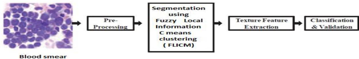
Fig 3.1. Overview of system using FLICM clustering
