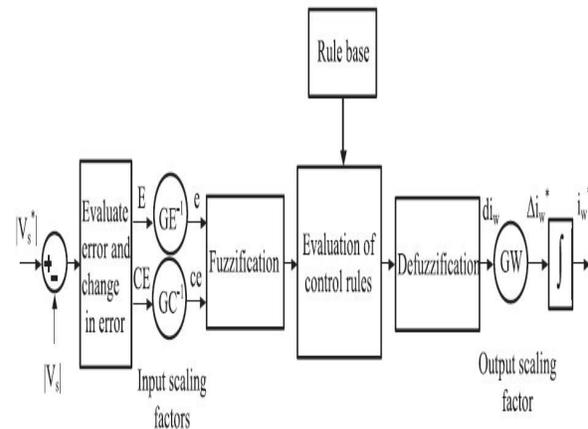
Fig 4 Block diagram of the FLC-1
