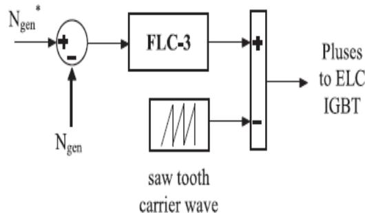
Fig 3 ELECTRONIC LOAD CONTROLLER (ELC)
