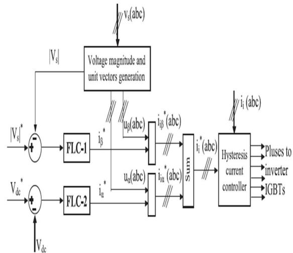
Fig 2 The Voltage controller
