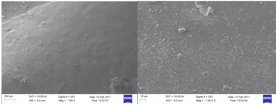
Fig. 3 : SEM of chitosan(a) and chitosan PAAM graft copolymer(b)
