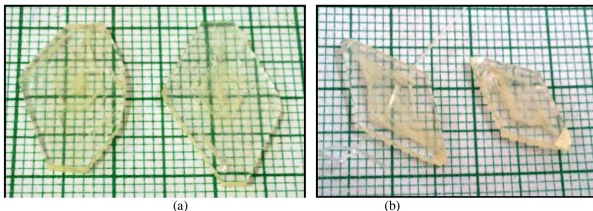
Fig. 1. Bulk Crystal grown by (a) Solvent evaporation method (b) Slow cooling method
