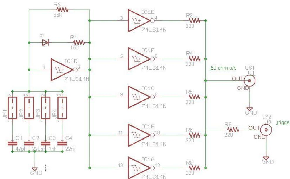
Fig 4 Circuit design for rectangular pulse wave generation with fast rise time.
