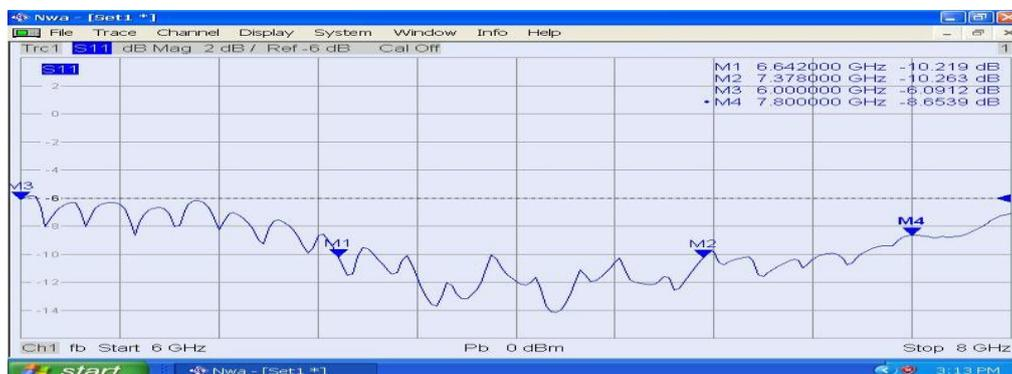
Fig 6 (a) Measured return loss of open ended 50- $\Omega$  SS probe at different frequencies
