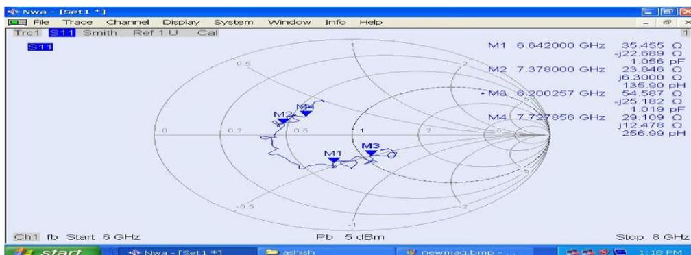
Fig 6(b) Smith chart for the calculation of characteristic impedance.
