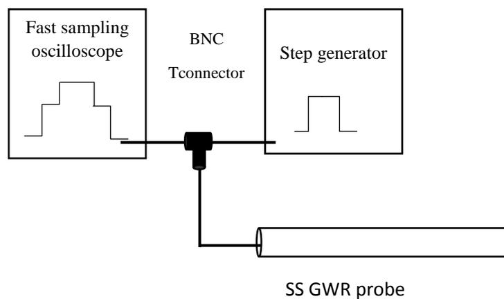
Fig 5 General laboratory setup for testing of signal generator and waveguide.
