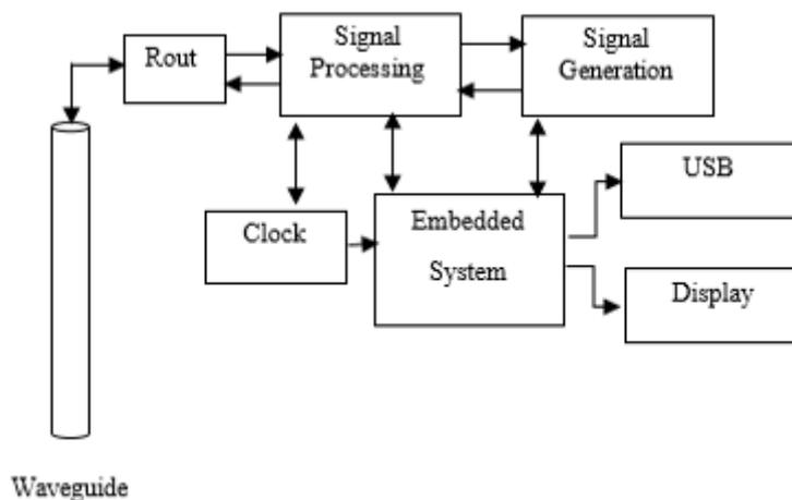
Fig 1 Architectural design of guided wave radar meter
