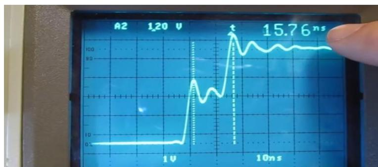
Fig 6 the resulting incident and reflected waveform at air-liquid interface
