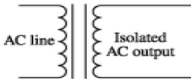
Fig.7. Isolation Transformer
