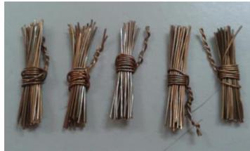
Fig. 2 Geometric details of twisted wire brush inserts
