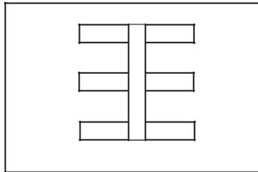
**Figure 2: Schematic diagram of complementary E-shaped DGS.**
