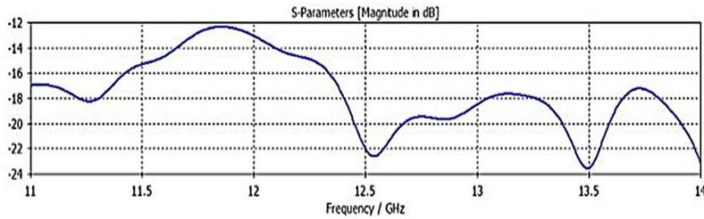
**Figure 3: Mutual coupling plot (S<sub>12</sub>).**
