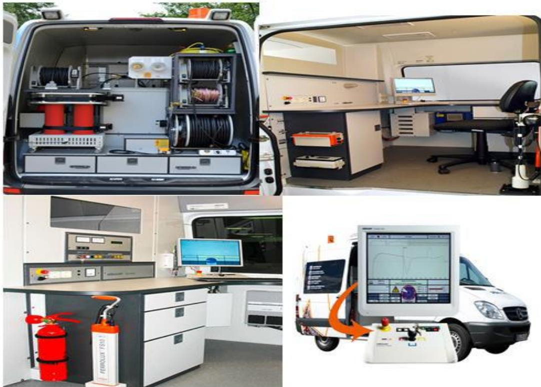
Figure 2: Centric system van for underground system cables faults.
