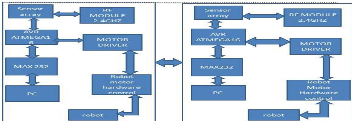
Figure 3: Prototype for the proposed system.
