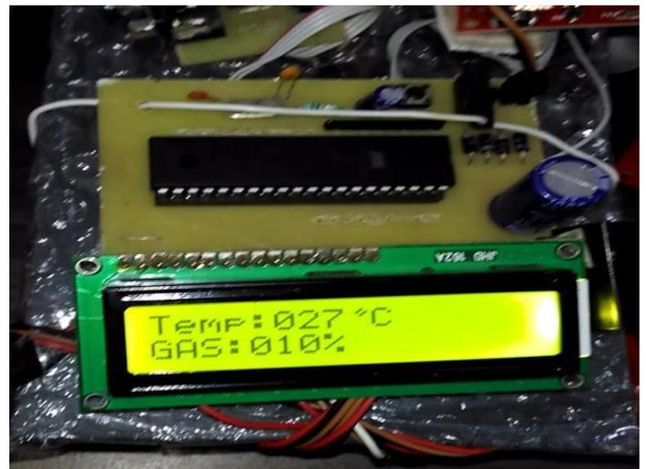
**Figure 4:** Final implementation of Air pollution monitoring Swarm robots.
