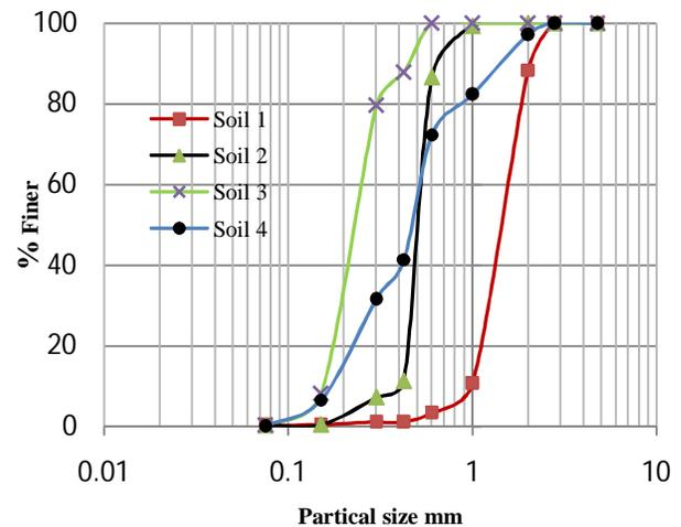
Fig. 3 Grain size distribution curves of soils used
