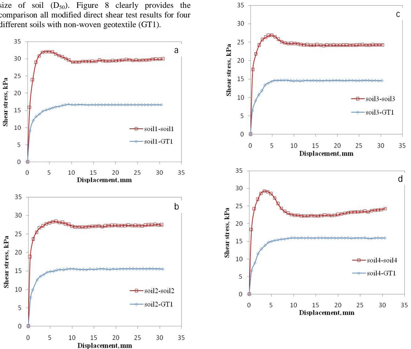
Fig. 7 Direct (soil-soil) and modified direct shear test
