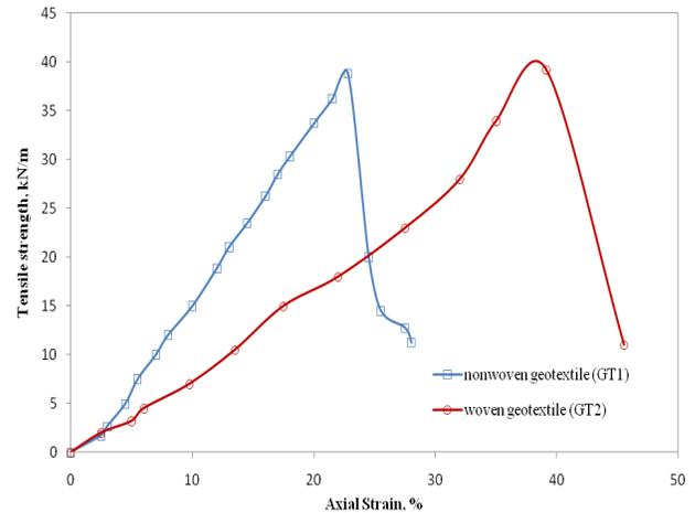
Fig. 6 Tensile load-strain behavior of GT1 and GT2
