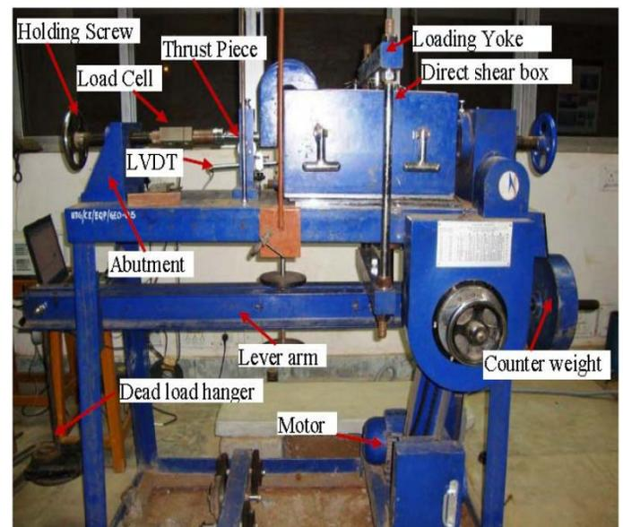
Fig. 1 Large direct shear box setup
