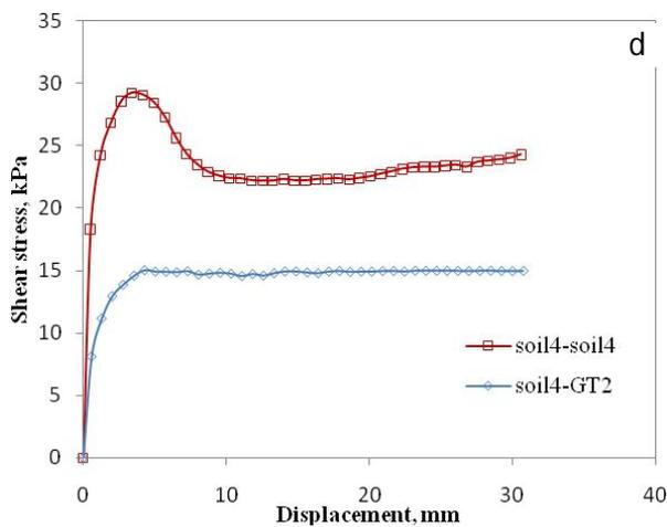
Fig. 9 Direct (soil-soil) and modified direct shear test (soil-GT) results of all soils with GT2
