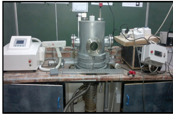
Figure 1. Pulsed laser deposition (PLD) system.
