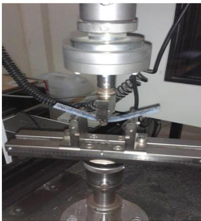
Fig.5 Flexural test fixture in Instron 3382 testing machine
