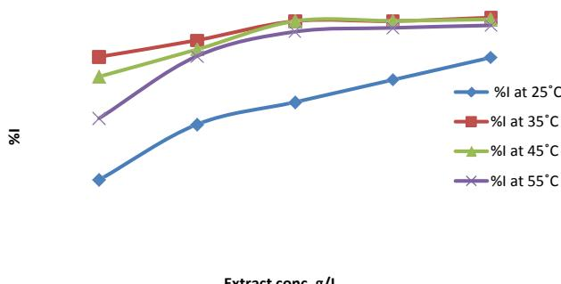
**Figure 3.** Inhibition efficiency versus (CD) extracts concentrations for aluminum in 1M NaOH at different temperatures after 1 h immersion time.
