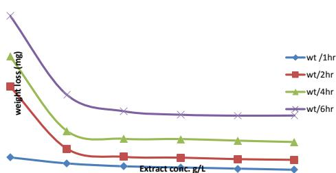
**Figure 1.** Weight loss variation of Al metal versus (CD) extract concentrations at 25°C in 1 M NaOH at different immersion times.
