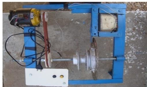
Fig 11 .Top view of the Fabricated Brake System
