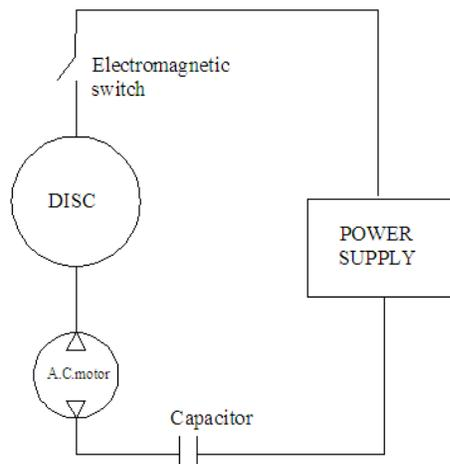
Fig.8 Working of Electro Magnetic Disc Brake
