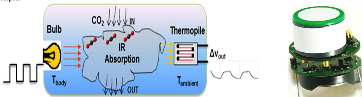
Figure 3: NDIR Gas Sensor Principle
