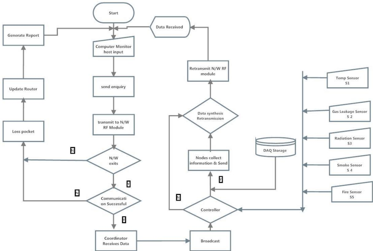
Fig 5: Software functional flow diagram
