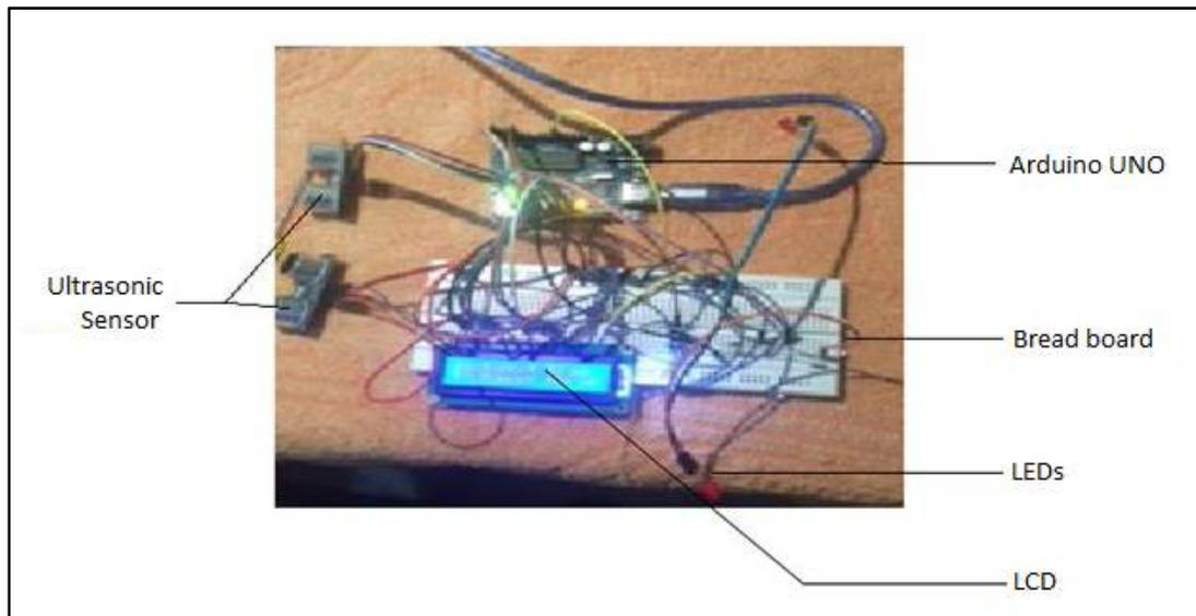
Fig. 4. Circuit for Tank Monitoring Module
