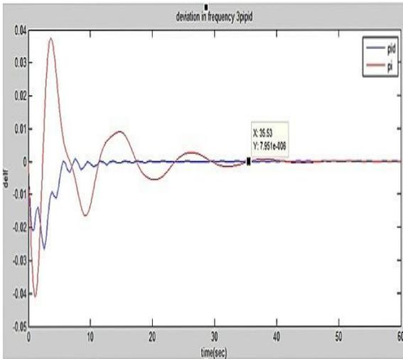
Fig. 5 Comparison graph of change in frequency of hydro-thermal power plant for PID to PI controller.
