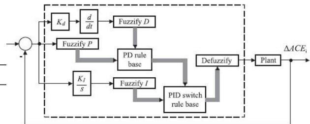
Fig. 2 The proposed multi stage fuzzy PID controller.
