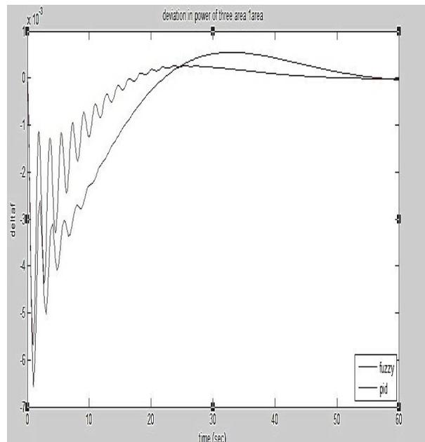
Fig. 7 Comparison graph of power deviation hydro thermal power plant with fuzzy PID and conventional PID.
