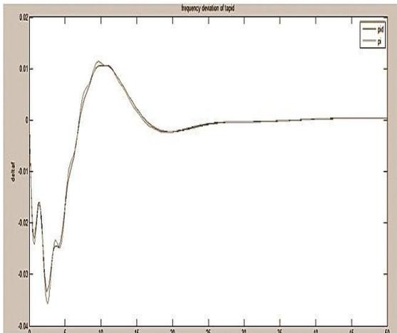
Fig 4: Comparison graph of thermal power plant for PID to PI controller.
