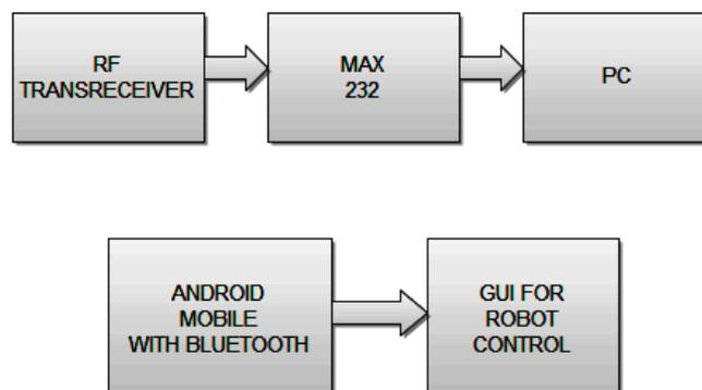
Fig.2. Control Section
