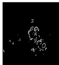
Initially the images were read and noise is removed using median filter shown in fig b). The above diagram fig.c) shows segmentation of both scanned images which are shown in white and black pixel. Then the preprocessed images will be taken as input for further module.
