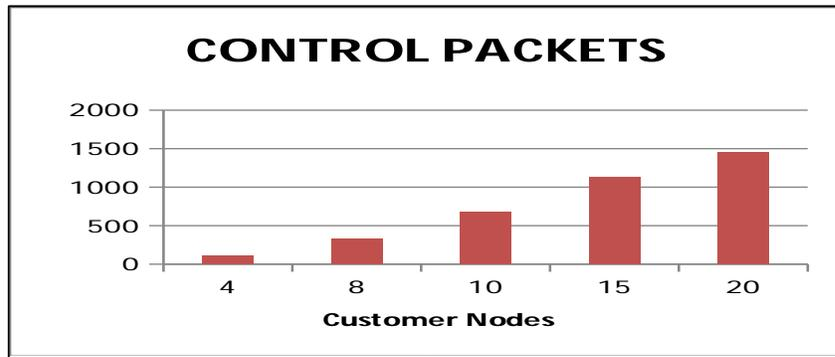
**Figure 5.B Customer nodes vs Control packets graph.** Here X-Axis denoted the number of Customer nodes and the Y-Axis denotes the number of Control Packets sent. The control packets forwarded increases linearly.
