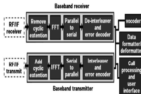
**FIGURE 2: A high-level block diagram of the transceiver baseband processing section in a 4G wireless design**
