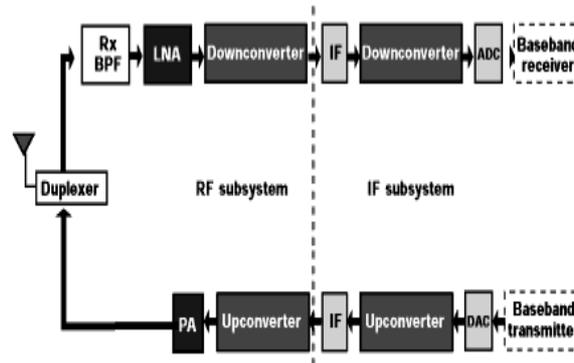
**FIGURE 1: A basic RF/IF block diagram showing a typical RF/IF section for a Transceiver**
