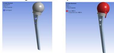
Fig No. 06 Loading and Boundary conditions
