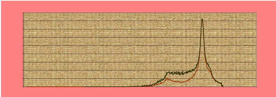
**Fig.2b)** Gamma ray spectrum of Water excited with the 59.54keV line. Geometry 45°/45° and Azimuthal angle =0°.The olive green line represents the vector model and the brown line represents the scalar model using MCSHAPE
