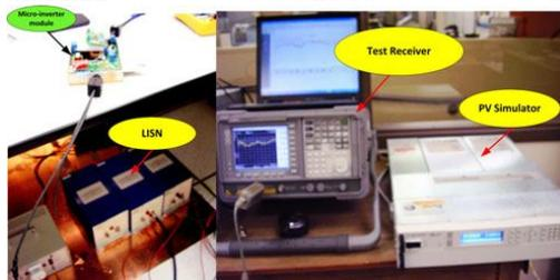
Fig. 14. Conducted emissions test setup.
