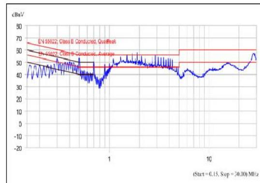
Fig. 16. Conducted emissions spectrum of the microinverter without EMI filters.
