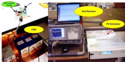
Fig. 14. Conducted emissions test setup.
