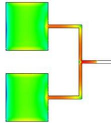
Fig. 1(d) Current Density of 2x1 Array
