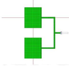
Fig. 1(c) Meshed Patch of 2X1 Array
