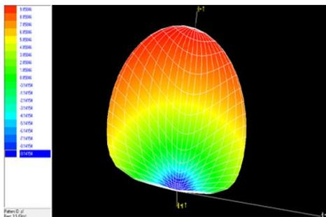
Fig.2 (c) 3-D Directivity Pattern of 2x1 Array
