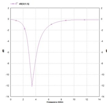
Fig. 2 (a) Return Loss characteristics of 2x1 Antenna Array
