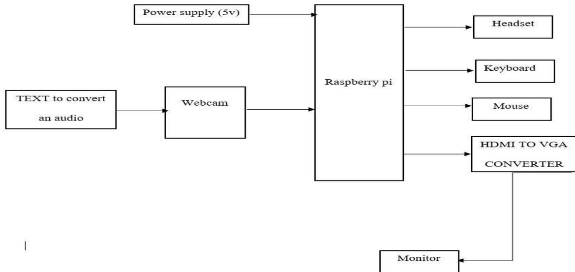
**Figure 2:** Block diagram of book reader with Raspberry pi.
