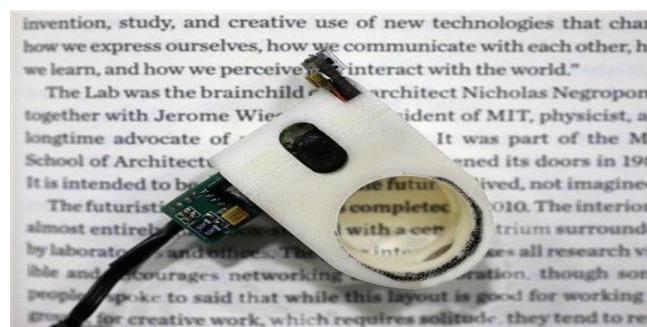
Figure 1: OCR based reader.
