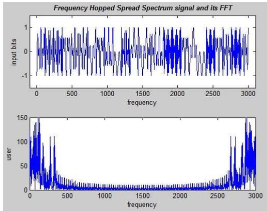
Figure 3 frequency hopping spread spectrum and its FFT
