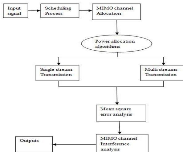
Fig 1Block diagram of Energy optimization in MIMO channel
