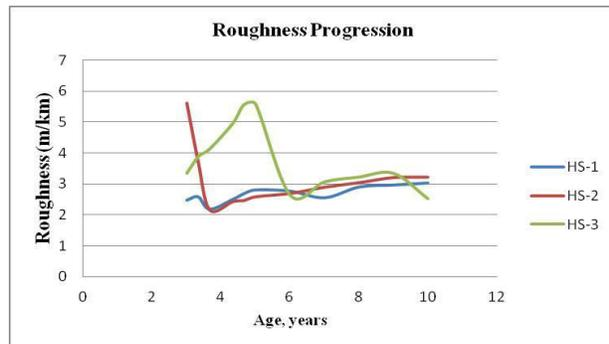
FIGURE 4 ROUGHNESS PROGRESSION IN VARKALA- KALLAMBALAM ROAD
