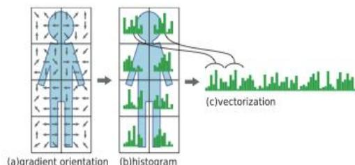
Figure 3.5 (a) (b) Overview of HOG calculation
