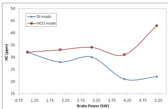
**Fig7.** Variation of hydrocarbon with brake power
