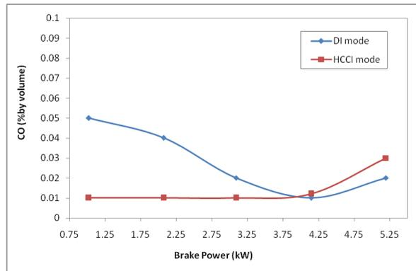
**Fig6.** Variation carbon monoxide with brake power
