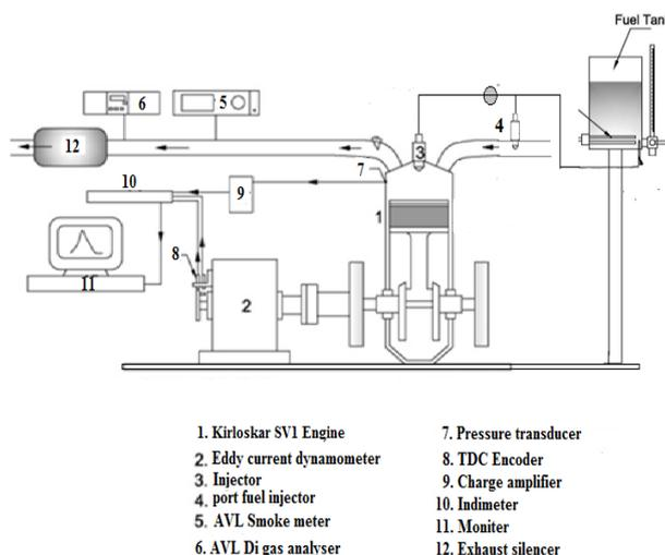
**Fig1.** Experimental setup of Kirloskar SV1 Engine
