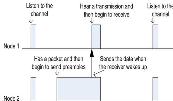
Fig. 4. Basic mechanism of LPL protocols.
