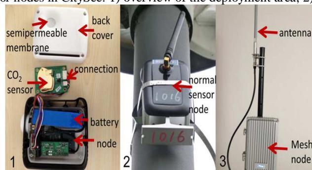
Fig. 2. Sensor nodes in CitySee: 1) CO sensor node, 2) normal sensor node, and 3) mesh node.
