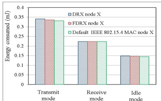
Fig.6. The effect of the DRX and FDRX schemes on the energy consumption.
