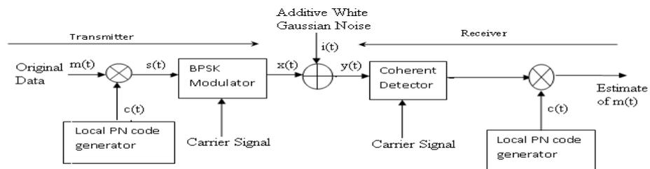
Fig.3 Block Diagram of DSSS Technique
