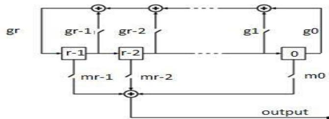
Fig.5 Block diagram of PN sequence
