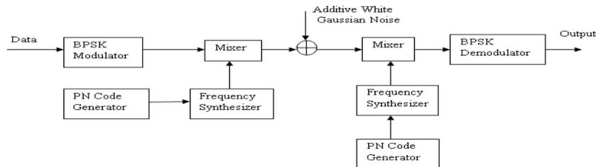
Fig.4 Block Diagram of FHSS technique
