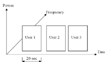
Fig.2 TDMA time slot allocation
