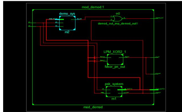
Fig 6.1 shows RTL view of DSS
