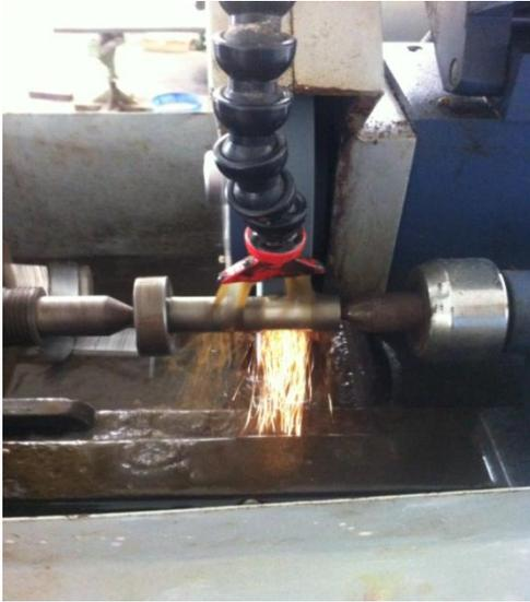
Fig. 1 Machining the mild steel rod with abrasive wheel during evaluation
