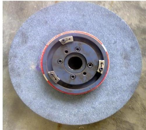
Fig. 2 Grinding wheel
