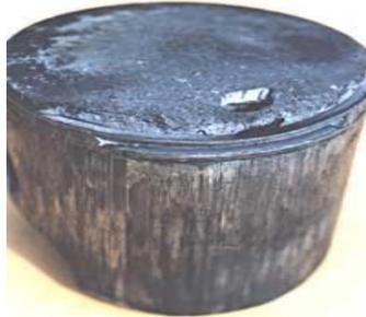
Fig.1. Burnt out blow hole on piston [2]
