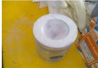
**Fig. 7.** TiO<sub>2</sub> Insulated piston
