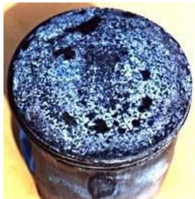
Fig.3. Melting of piston crown [2]
