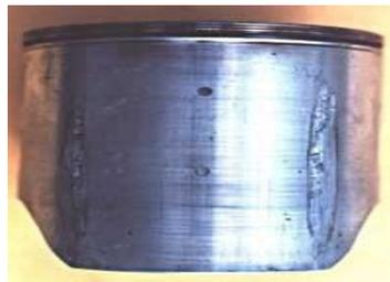
Fig.2. Four corner seizure on piston [2]
