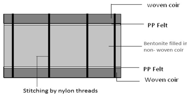
Fig.3.1. Schematic diagram Sample 1
