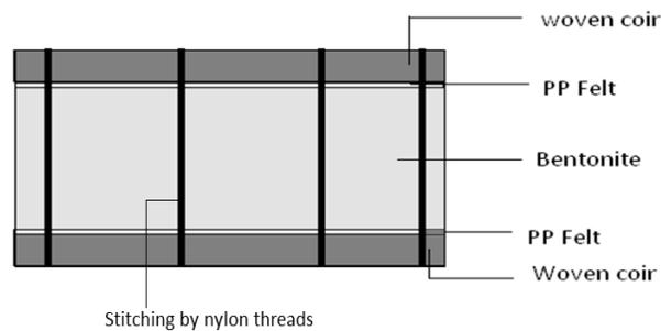
Fig.3.2. Schematic diagram Sample 2
