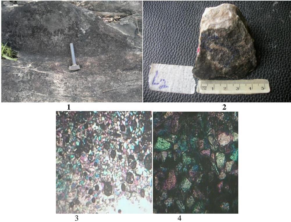
1. Calcareous Sandstone, quarry site at location .2 along Amasiri-Ozara Ukwu Road: Calcareous Sandstone, quarry site at location 2 along Amasiri-Ozara Ukwu Road. 3 & 4 Photomicrographs of Buchite hornfels,. Note speckes of magnetite minerals and a granoblastic mosaic of quartz and feldspars, with web texture.
