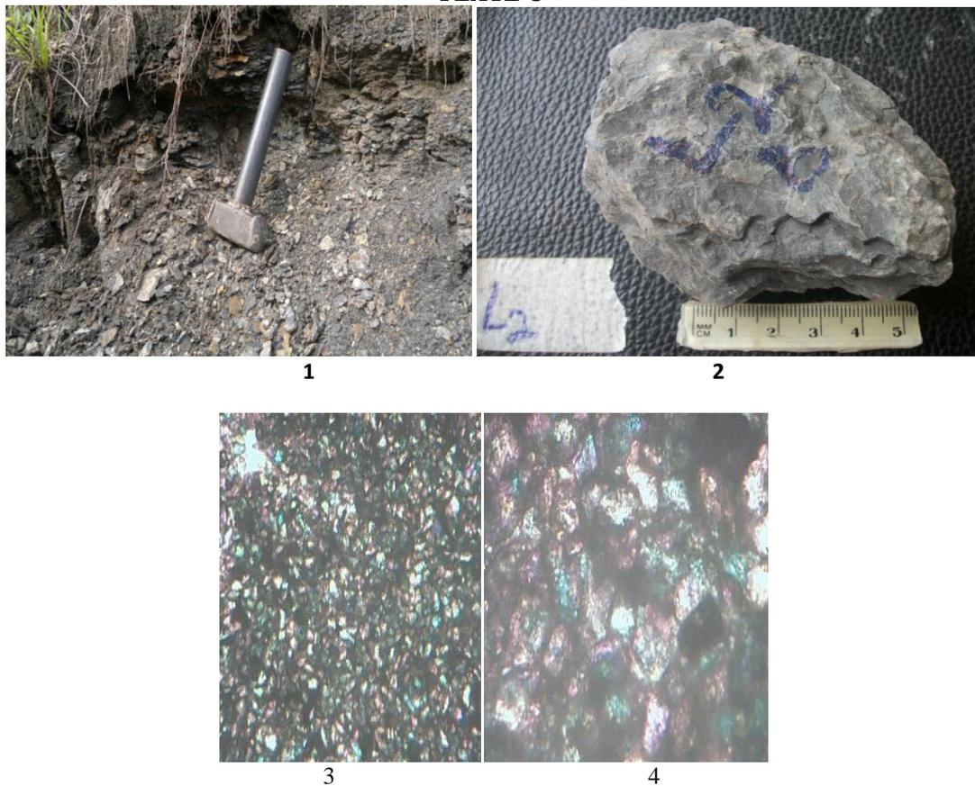
1: Slate, quarry site at location along Amasiri-Ozara Ukwu Road.:2 Hand specimen of Slate.: 3&4 Photomicrographs. Note porphyroblasts of sericitized chialstolite enclosed in a matrix of biotite, graphite and quartz.
