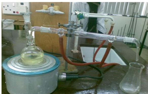
Figure 2. Cold Extraction of walnut oil from petroleum ether.
