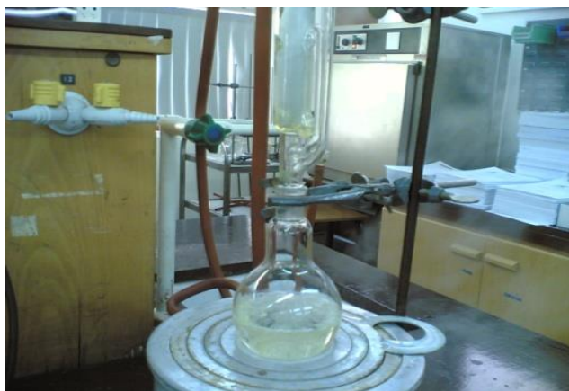
Figure 3. Cold Extraction of walnut oil from petroleum ether
