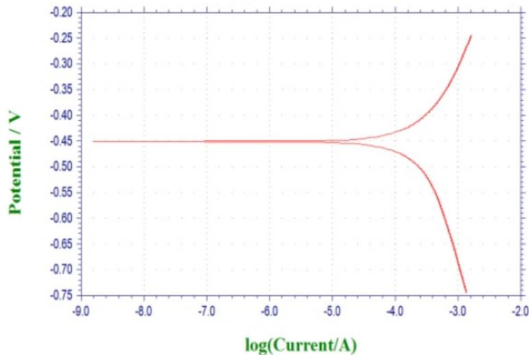
Figure 4. Tafel polarization curve in 0.75 N HCl.
