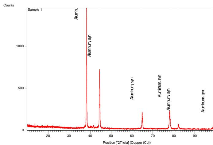
Figure 8. X-ray diffraction pattern Spectrum of Al 2024 alloy.
