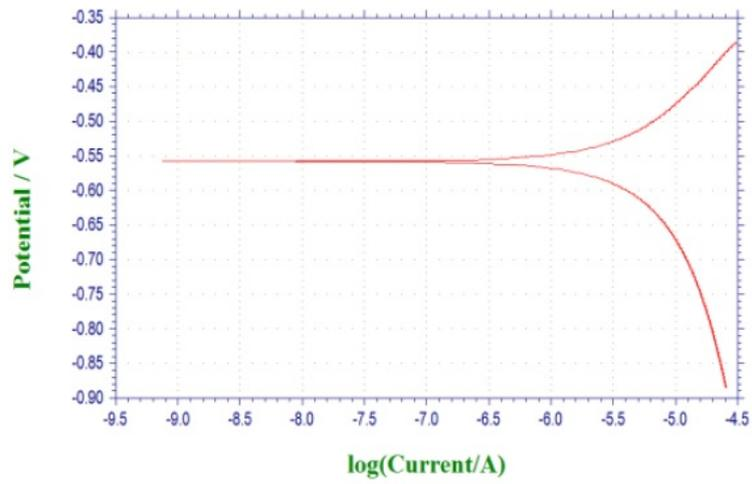
Figure 2. Tafel polarization curve in 0.75 N HCl.
