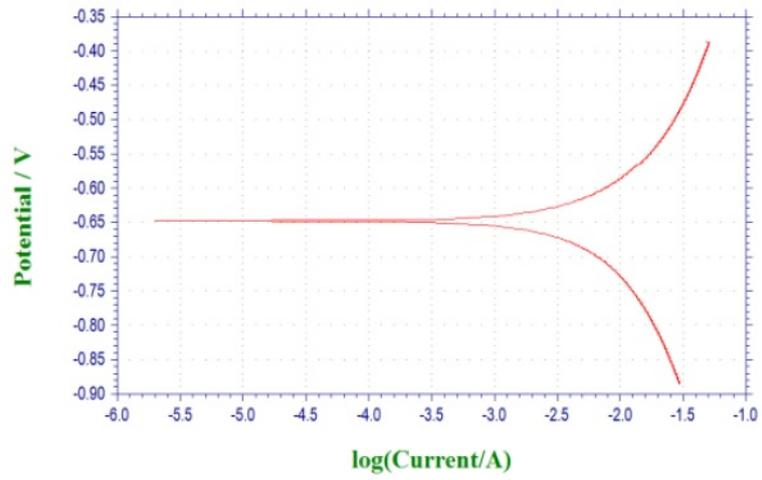
Figure 1. Tafel polarization curve in 1 N HCl.
