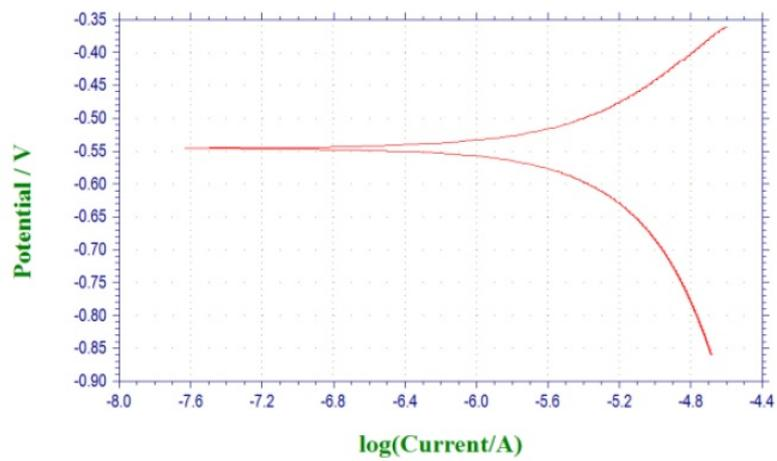
Figure 3. Tafel polarization curve in 1 N HCl.
