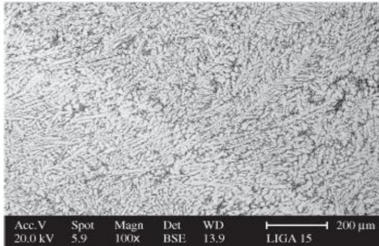
Figure 6. Al 2024 alloy before corrosion test.
