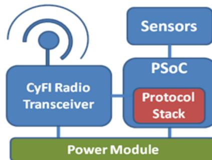
Fig.1. Blocks of wireless sensor node
