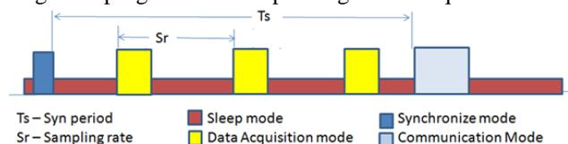
Fig.2 Proposed wireless sensor node's operations mode
