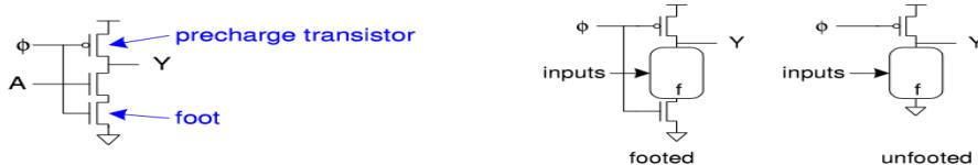
Fig.1.Logic diagram of Footed Technique
