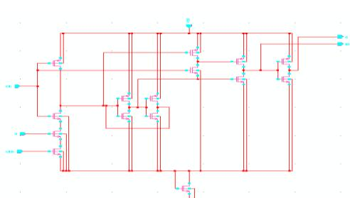
Fig.7.Schematic Diagram of Proposed DDFF with footed logic
