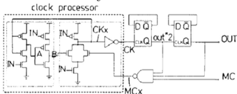
Fig.2. Schematic diagram of circuit of divide-by-4/5
