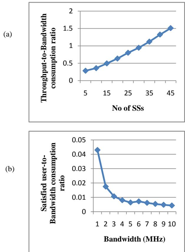
Fig. 4 (a) Network throughput-to-bandwidth consumption ratio and (b) Users-to-bandwidth consumption ratio
