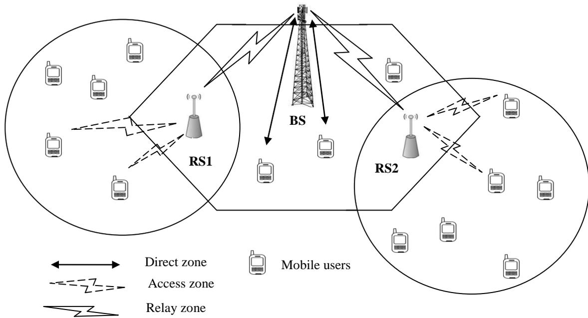
Fig. 1. Structure of WiMAX relay network
