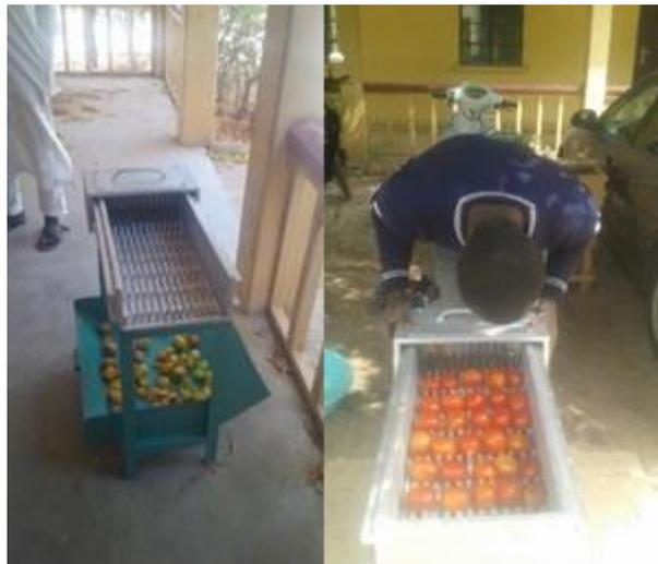
Figure 1: Modified and Old manual tomato slicing machines.
